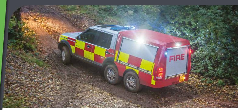
The all-new Specialist Utility Vehicle 600 (SUV 600) has taken a production standard Land Rover Discovery 4x4 and adapted it for use in the Emergency Services and wider utility sectors.
